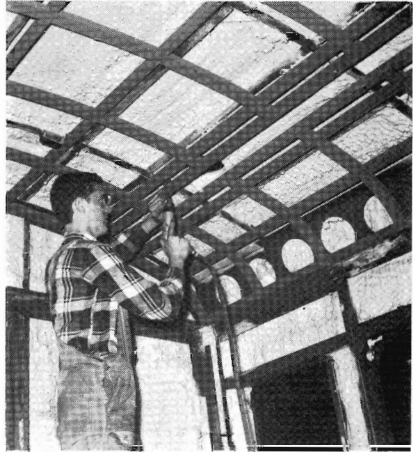
HARRIS CARRIAGES: At Newport Workshops, one of the 10 Harris motor carriages that are being built, is test-lined with polyurethane foam.
