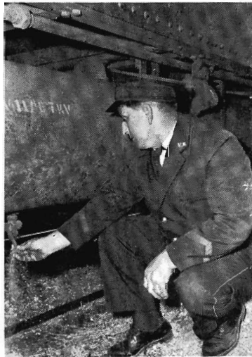
A News Letter photographer visiting Ultima, found Rail Motor Driver D. Garcia draining the air reservoir of the rail motor. Mr. Garcia joined the Department in 1953, and has been at Ultima for the past six years. Before that he worked at Echuca. He is president of the local branch of the R.S.L., and a keen golfer.
